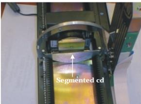
You will need a section of an old CD (see segmented disc below) to view Bow Arm alignment.
