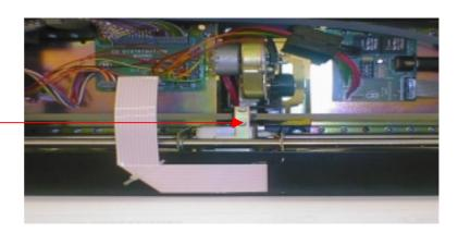
Place one of the count position disc slots is in the middle of the count opto. Display '2' led (decimal point) should be illuminated.
