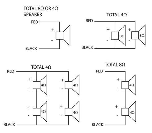
Each channel on the speaker matching pad should be connected independently. Under no circumstances should a single ground line be used to connect all the speakers back to the pad, doing so will cause the amplifier to enter a fault condition.
