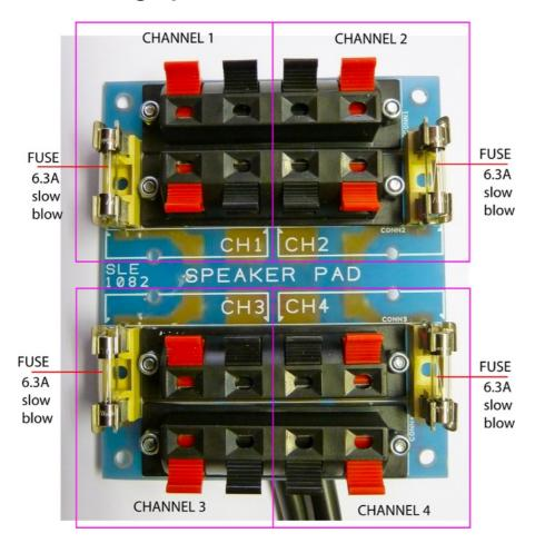
Each channel can take a minimum load of  $4\Omega$ .
