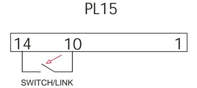
When the switch is closed the jukebox will play BGM on a permanent basis until the switch is opened again. The discs selected for BGM will be the band of discs previously programmed into Menu 5 at levels 3 and 4.
